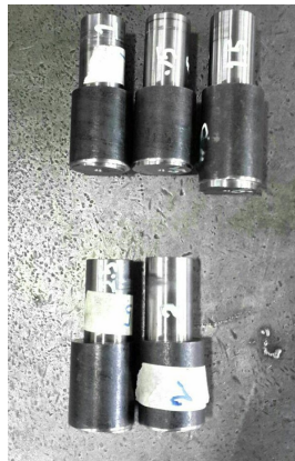
Fig. 4. Eccentric AISI 4340 tools for applying loads with certain amplitudes
