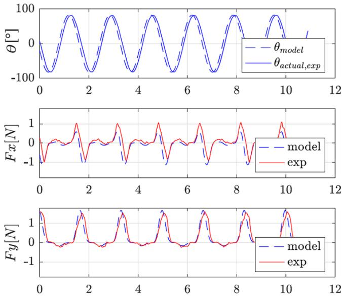
**Fig. 7.** Ease of design. The simplicity of the flapped-paddle and the low impact of the hydrodynamic artifacts, enabled us create high-fidelity models. The above figure shows the lateral and longitudinal forces, with  $l_0 = 3$  cm,  $l_1 = 10$  cm,  $w = 6$  cm,  $w_r = 0.6$  cm, obtained using models (Eq. (3)) and experiments
