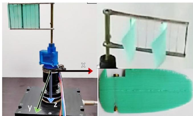
**Fig. 3.** Flipper mount (left) and structure (right). The symmetry in the structure of the conventional flipper (right, bottom) cancels the lateral drag force; the flapped-paddle (right, above) opens fully in the recovery-stroke and closes in the power stroke; there is little impact on mounting on the test-plate (left)
