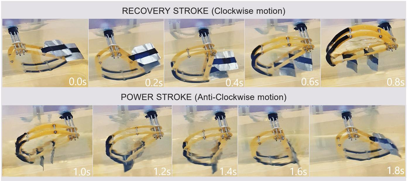
**Fig. 5.** Responsive design. Note that in aquatic environments the flaps rapidly close to increase the utilization of the power stroke cycle (top). In the recovery stroke, the flaps rest along the structure of the flow, minimizing drag (bottom)
