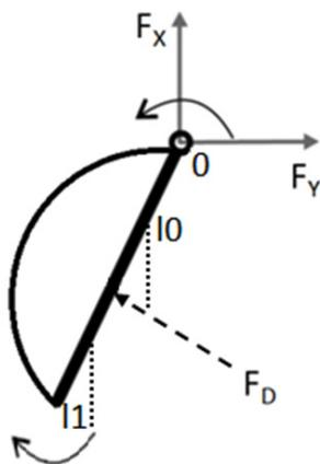
**Fig. 6.** Force diagram. Drag-forces generated during oscillation in an aquatic environment under low inflow conditions. Note that the flaps rotate in opposite orientation to the leg rotation
