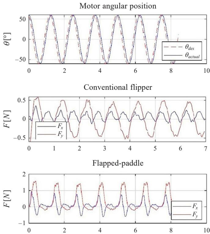
**Fig. 2.** Asymmetry improves propulsive efficiency. The symmetry in the lateral drag force ( $F_y$ ) for the conventional flipper (top) results in zero average force in an aquatic environment. Notice that the lateral drag force for the flapped-paddle is suppressed in the recovery stroke, thus maximizing propulsive efficiency because  $F_x < F_y$
