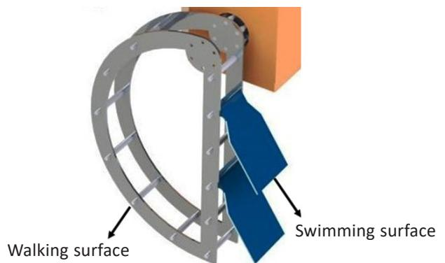
**Fig. 4.** Multi-regime, composite Fin-Leg. The flapped-paddle can be easily integrated into a variety of mechanical structures to enable both terrestrial and aquatic locomotion. In the above figure, the flapped-paddle has been integrated into the RHex Leg [13]
