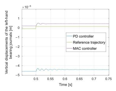
**Fig. 7.** Vertical displacements of the left-hand bearing journals obtained using the control algorithms being tested
