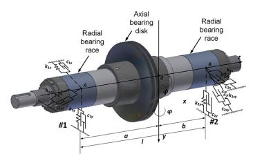
**Fig. 1.** Rigid-body model of the rotor shaft of high speed rotating machine suspended on active magnetic bearings
