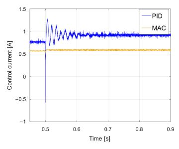
Fig. 9. Time histories of the left-hand bearing current responsible for controlling vertical motion obtained using the control algorithms being tested
