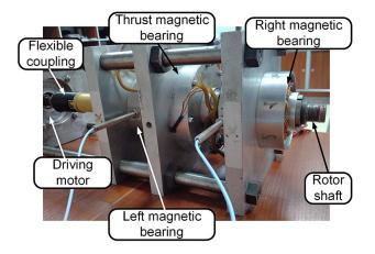
Fig. 5. The magnetic suspension system of the laboratory rotor-shaft
