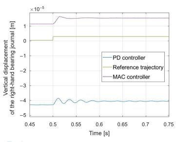
**Fig. 8.** Vertical displacements of the right-hand bearing journal obtained using the control algorithms being tested
