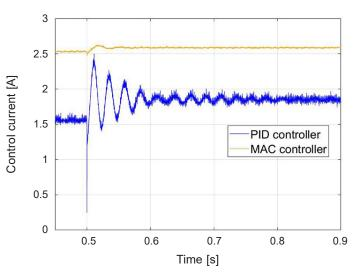
Fig. 10. Time histories of the right-hand bearing current responsible for controlling vertical motion obtained using the control algorithms being tested
