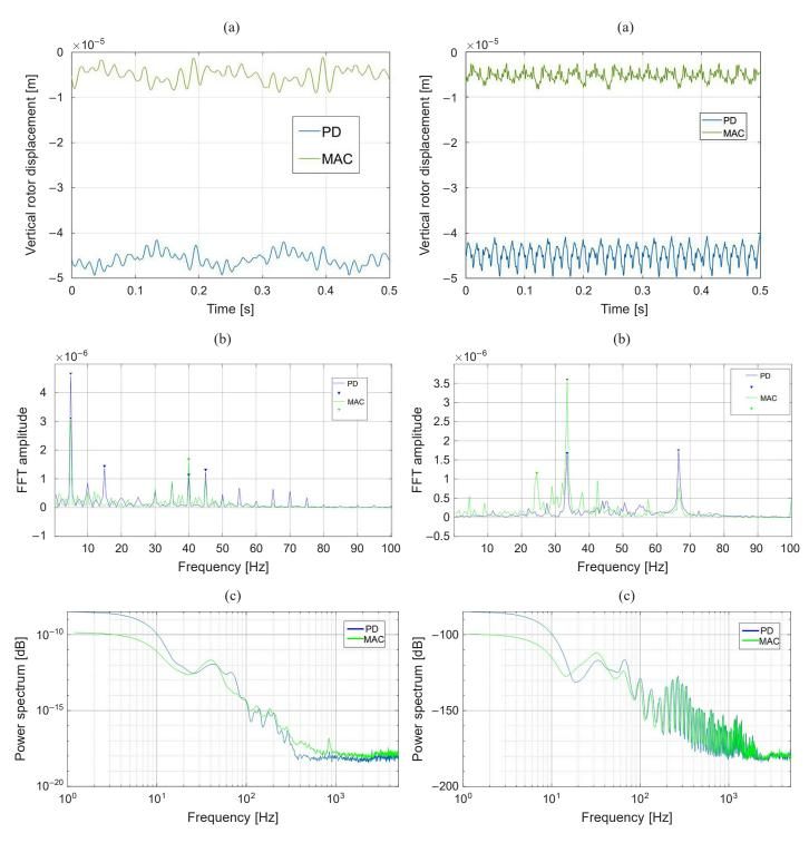
Fig. 11. Vertical displacements of the left-hand bearing journal obtained at the rotational speed of 300 rpm, a) time histories, b) FFT amplitude, c) power spectrum
