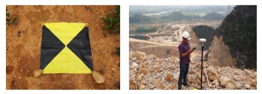
Fig. 2. GCP marks and their coordinates measured by GNSS/RTK
