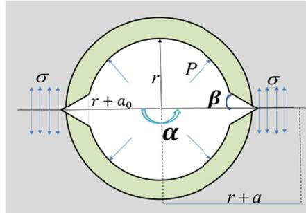
Fig. 2. Principle of Bilateral Cumulative Tensile Explosions
