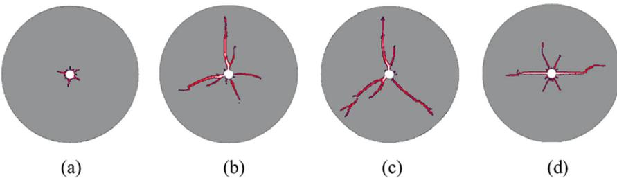
Fig. 4. Comparison of ordinary blasting and BCTE:
