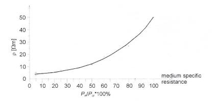
Fig. 2. Diagram of relations of power of recorded impulses of electromagnetic waves and the medium specific resistance
