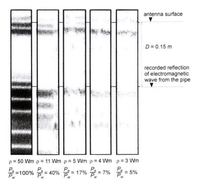
Fig. 1. Echograms of variations of power of recorded signals reflected from the pipe of 0.1 m diameter, located in media of various specific resistance
