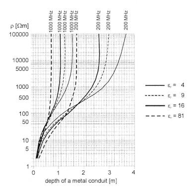
Fig. 3. The scope of measurements of depth of a metal conduit of diameter  $\phi = 0.1$  m with the use of geo-radar antennae 200 and 1000 MHz in media of various specific resistance  $\rho$  and dielectric constant  $\varepsilon_r$
