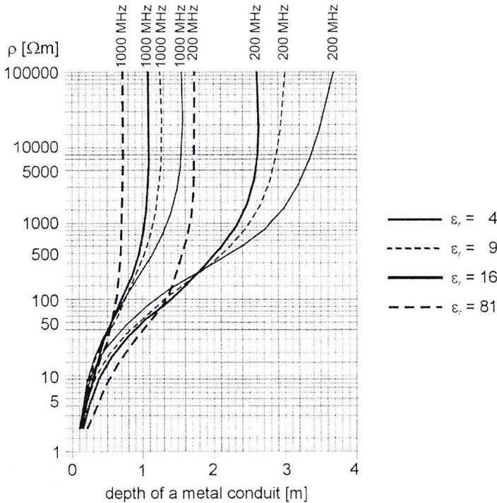
Fig. 3. The scope of measurements of depth of a metal conduit of diameter  $\phi = 0.1$  m with the use of geo-radar antennae 200 and 1000 MHz in media of various specific resistance  $\rho$  and dielectric constant  $\epsilon_r$ ,
