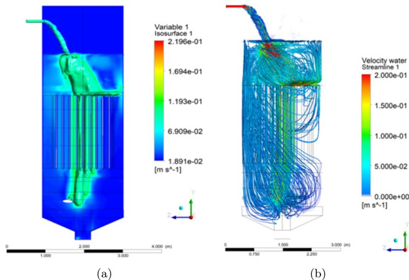
Figure 3: Numerical evaluation of the flow in the fermenter: a) velocity isosurface – quality view of the main mixing area and where the highest velocities occur; b) streamlines – view of the recirculation zone.
