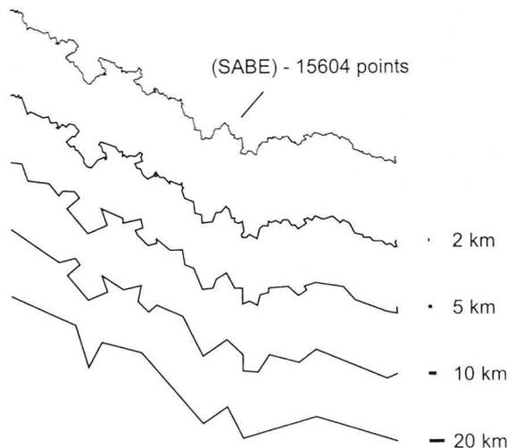
Fig.1. Generalisation of the southern frontier of Poland with the use of Douglas-Peucker algorithm
