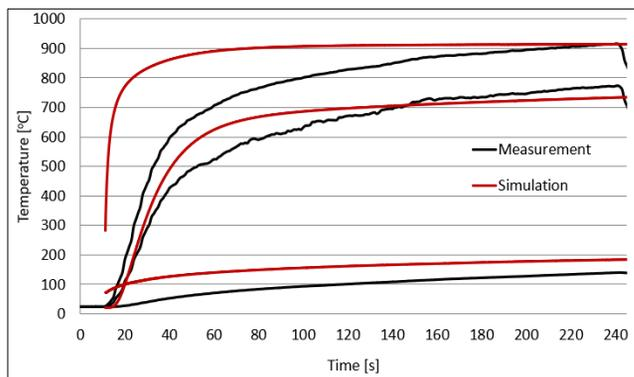
Fig. 5. Temperature change curves in the combustion chamber, simulation, and measurement results during tests
