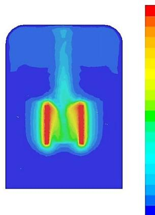
Fig. 2. Temperature field in the measuring chamber – simulation results
