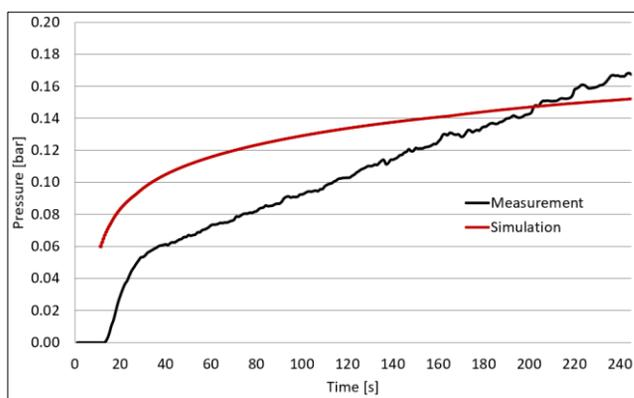
Fig. 6. Pressure changes curves in the combustion chamber, simulation, and measurement results during tests
