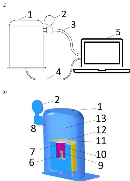
Fig. 1. Measuring stand. a) workstation's schematics; b) view in the section of the combustion chamber.
