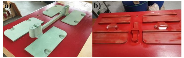
Fig. 7. Molding in OMEGA device: a) upper model plate for molding; b) bottom plate for the molding
