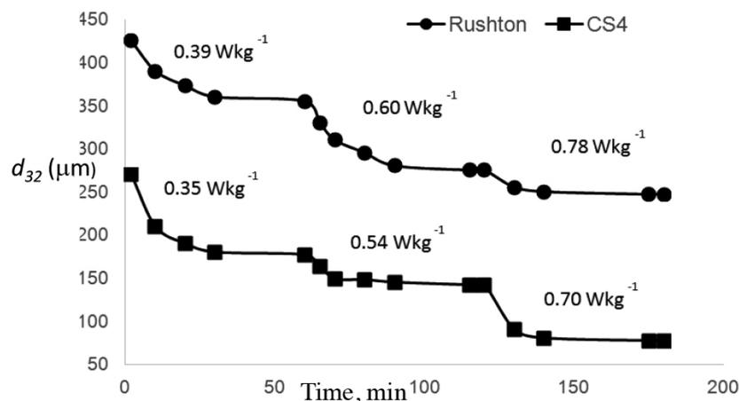
Fig. 4. Sauter mean drop size transients for the RT and CS 4 for the 100 cSt silicone oil as a function of the specific power input,  $P/M$  W/kg (mean specific energy dissipation rate,  $\bar{\epsilon}_T$ , W/kg), for the Rushton turbine and CS 4 impeller
