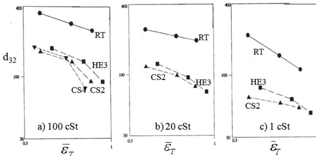
Fig. 3. Steady state Sauter mean drop diameter,  $d_{32}$ , versus specific power input,  $P/M$ , W/kg, ( $\equiv$  mean specific energy dissipation rate,  $\bar{\epsilon}_T$ ) for the different impellers studied: a) 100 cSt; b) 20 cSt; c) 1 cSt
