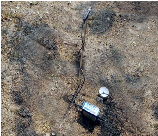
Fig. 11. Seismograph measuring the ground vibration
