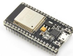
Fig. 14. ESP32 Board
