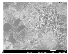
Fig. 9. Microstructure of DI-CuW3 ductile iron
