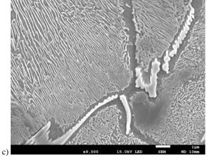
Fig. 8. Microstructure of DI-CuW2 ductile iron
