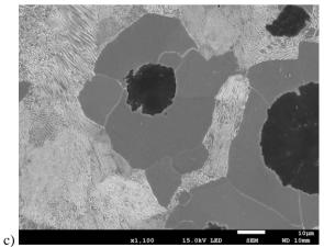
Fig. 6. Microstructure of DI-Cu ductile iron
