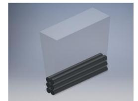
Fig. 5. YII shape casting with specimens for metallographic and mechanical properties examinations
