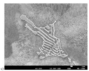
Fig. 7. Microstructure of DI-CuW1 ductile iron
