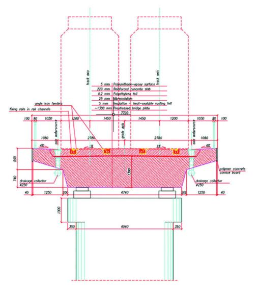
Fig. 2. Diagram of the cross section of the tramway road in Rakoczego St., Gdansk [10]
