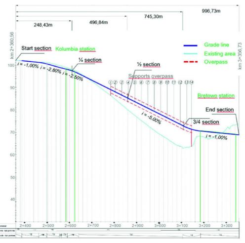
Fig. 3. Diagram of the vertical alignment of the analysed section of the tramway road in Rakoczego St., Gdansk [10]
