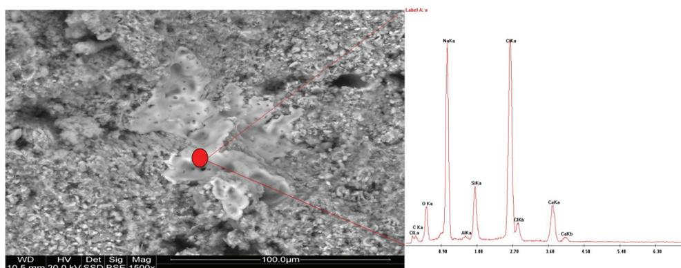
Fig. 2. Salts crystallizing in the light opoka-rocks space from Kazimierz Dolny. SEM/EDX
