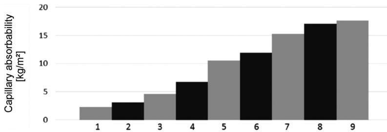
1 – Concrete with density  $2300 \text{ kg/m}^3$ , 2 – The Krasnobród opoka-rock, 3 – The Wola Komborska sandstone, 4 – The Bochothnica opoka-rock, 5 – Calcareous-ceramic mortar, 6 – Fine grained sandstone, 7 – The Kazimierz opoka-rock, 8 – The Annapol opoka-rock, 9 – Ceramic brick
