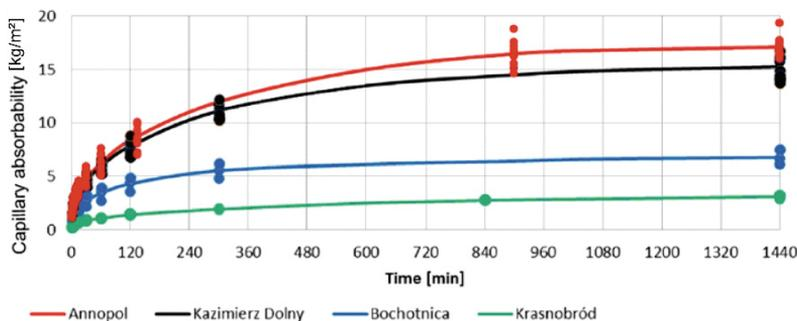
Fig. 6. Capillary absorptivity of the studied opoka-rocks in time
