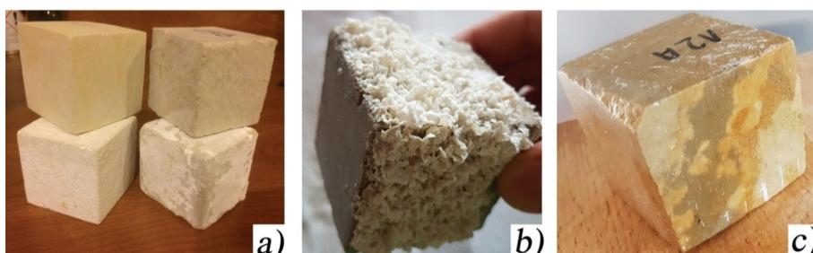
Fig. 1. Appearance of the opoka-rocks following the acid test: a) light opoka-rock on the left and heavy opoka-rock on the right after soaking in acidic solution, b) heavy opoka-rock – salt precipitation, c) light opoka-rock – color change on the surface
