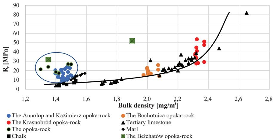
Fig. 7. Relationship between compressive strength and bulk density of rocks (own elaboration and based on [3, 12, 30])
