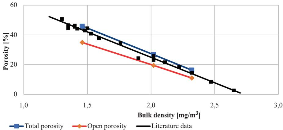
Fig. 3. Relationship between porosity and bulk density of the opoka-rocks
