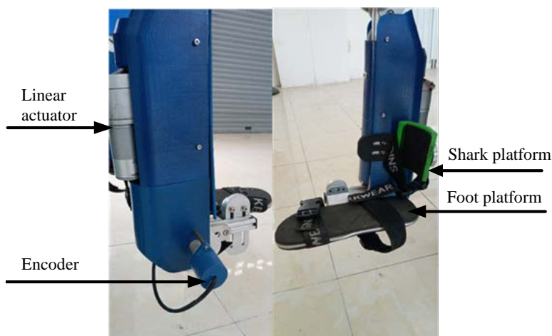
Fig. 7. Prototype of the ankle rehabilitation device
