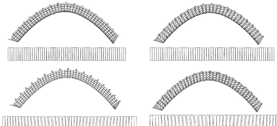
Fig. 8. Program output and unrolled panel rows. Top plots were produced with the first version of the algorithm, bottom with the second. The left column shows straight panels, right column panels rotated by 15 degrees. Number of panels: top-left = 240, bottom-left = 258, top-right = 204, bottom-right = 222
