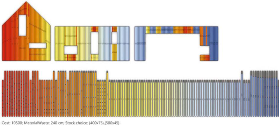
Fig. 9. Exemplary program output. Top: façade plans with cladding. Bottom: stock material required to make the cladding. The source stock planks are numbered and colour coded
