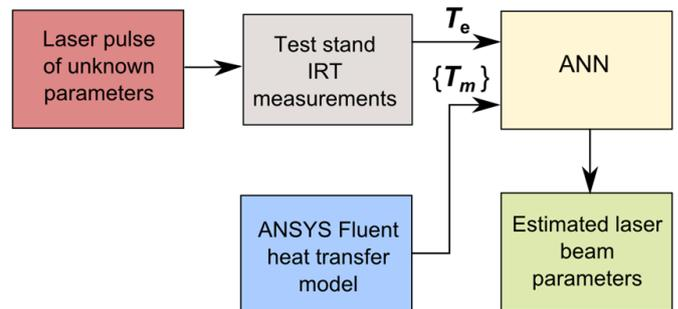
Fig. 3. The schematic of the intended method
