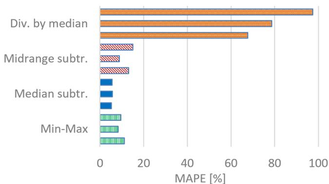
**Fig. 11.** Comparison of estimation errors for various methods of input data transformation (3 results per method shown individually)
