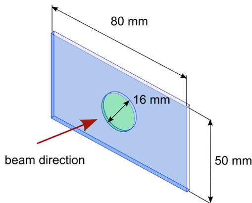
Fig. 2. The geometry of the laser-heated plate
