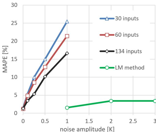
**Fig. 13.** Dependence of the ANN parameter estimation error on the number of inputs and the level of noise for the finally chosen topology X-1000-1000-3 (performance of the alternative LM method is also shown for comparison)
