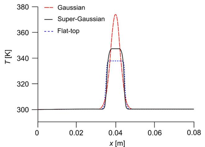
**Fig. 1.** Profiles of temperature at the surface of thin aluminum plate obtained by heating it with a high-power laser beam of three basic spatial energy distributions – Gaussian, super-Gaussian and flat-top (adopted from [9])
