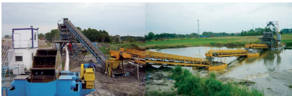
Fig. 3. Wet open-cast extraction of sand (primary commodity) and amber (associated commodity), “Przeróbka SL” deposit in Gdańsk. Phot. K. Twardowski, 2016 (Baltex Minerale) (taken from Kowalska et al. 2018)
