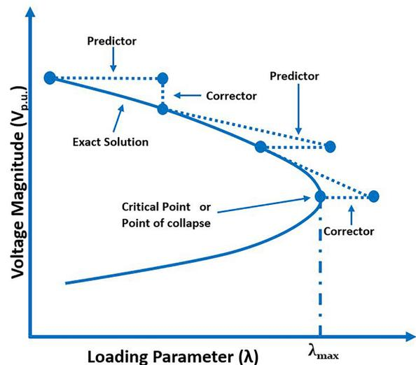
Fig. 2. Predictor-corrector approach used in the CPF
