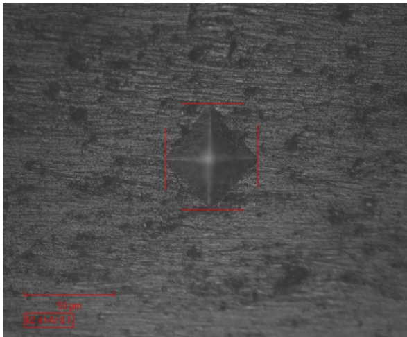
Fig. 5. Micrograph showing the microhardness of the fabricated specimen across the cross-section
