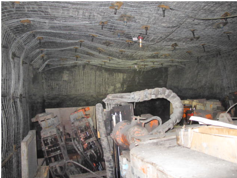
Fig. 5. Bolter Miner 12CM30 and the rock bolt support in the Budryk mine
