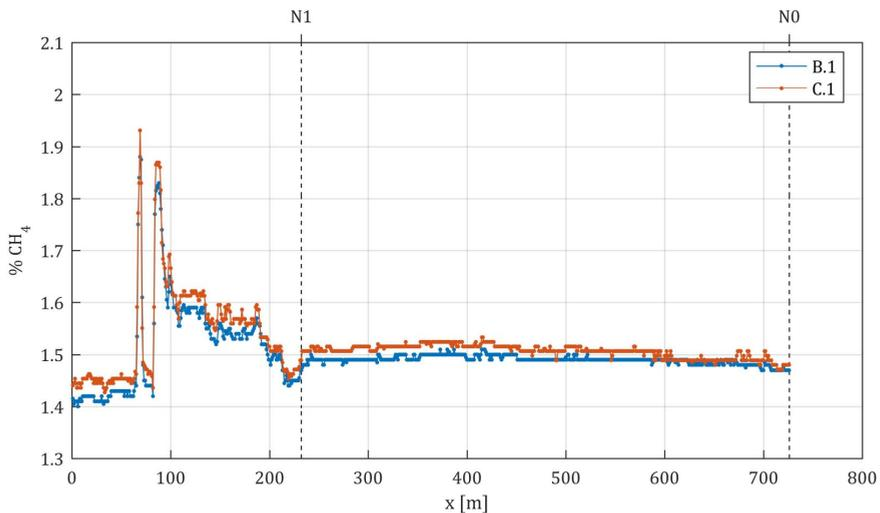
Fig. 9. Waveforms of methane concentration along the longwall gallery (506)
