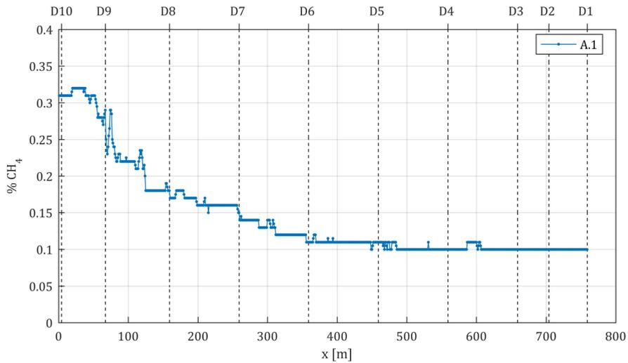
Fig. 8. The course of methane concentration along the ventilation road (512)
