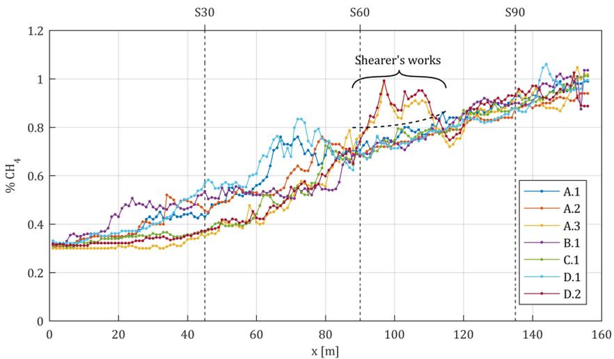
Fig. 7. The course of methane concentration along the longwall
