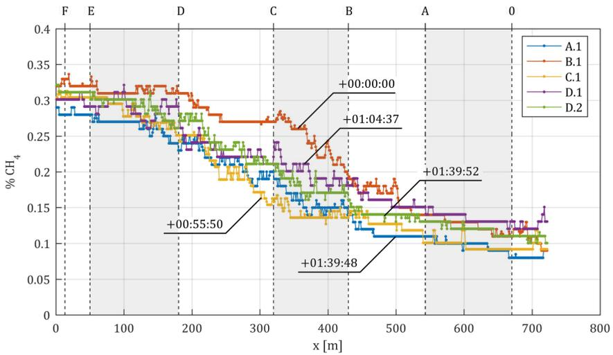
Fig. 6. Waveforms of methane concentration along the main gate (510)
