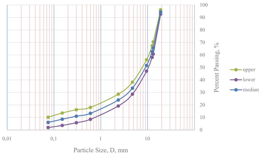
Fig. 5. The New Aggregate gradation 'S' curve
