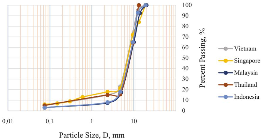
Fig. 3. Ordinary Aggregate gradations for porous asphalt for all five asean countries
