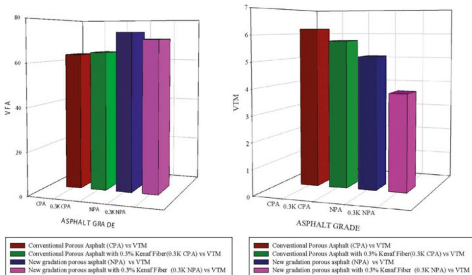
Fig. 7. Volumetric properties VFA and VTM of porous asphalt mixtures
