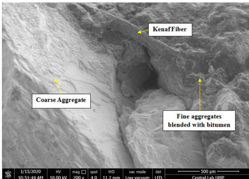
Fig. 2. SEM Images of PA modified with Kenaf Fiber
