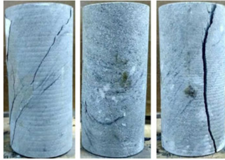
Fig. 12. Rock samples obtained on-site and post-fracture characteristics
