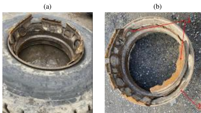
Fig. 4. The failed wheel with the damaged rim: (a) with a tire; (b) without a tire, 1 – fragment of the damaged rim, 2 – fragment of the rim that is free from damage
