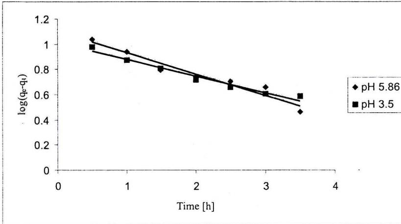
Fig. 5. Kinetic of Cr(VI) removal on ion-exchange resin Amberjet 4200 Cl
