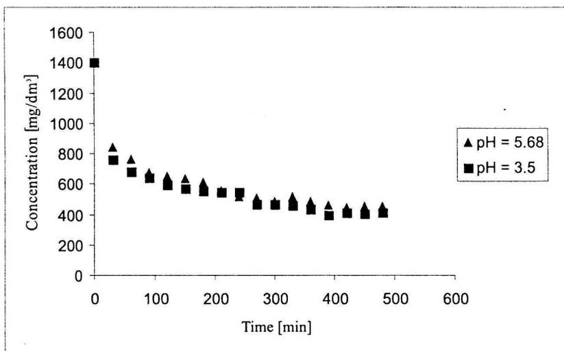
Fig. 4. Cr(VI) removal kinetic curve in flow condition
