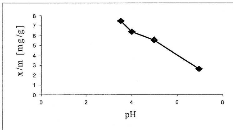
Fig. 2. Effect of pH on sorption capacity of GFH
