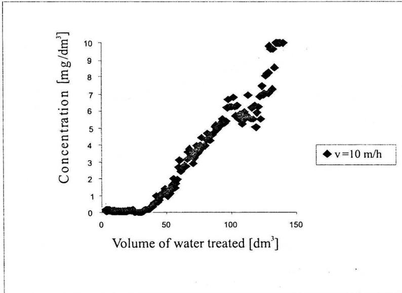
Fig. 7. Final concentration of Cr(VI) after sorption on GFH column
