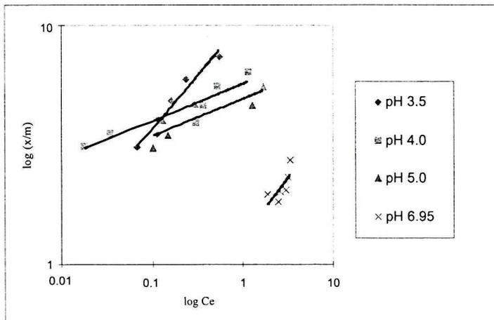
Fig. 1. Correlation between final concentration of Cr(VI) and  $x/m$  ratio on GFH at various pH
