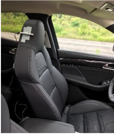
Fig. 6. In-vehicle background noise recording.
