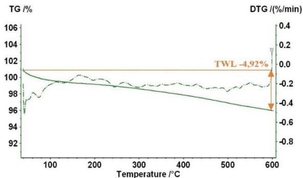
Fig. 3. TG / DTG curve measured for sample no. 1
