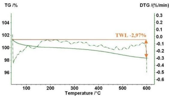
Fig. 17. TG / DTG curves measured for sample no. 7 (after biodegradation process)
