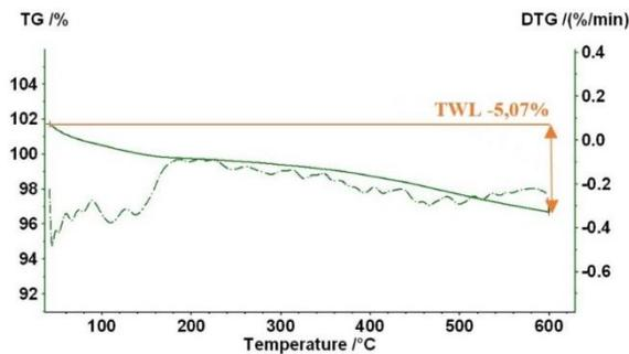
Fig. 15. TG / DTG curve measured for sample no. 5 (after biodegradation process)
