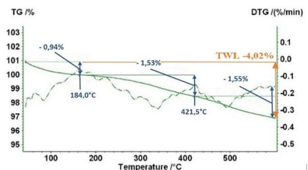
Fig. 8. TG / DTG curves measured for sample no. 6
