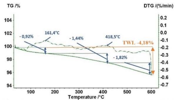
Fig. 4. TG / DTG curves measured for sample no. 2
