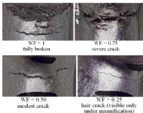
Fig. 5. The WF for various tearing types [42]
