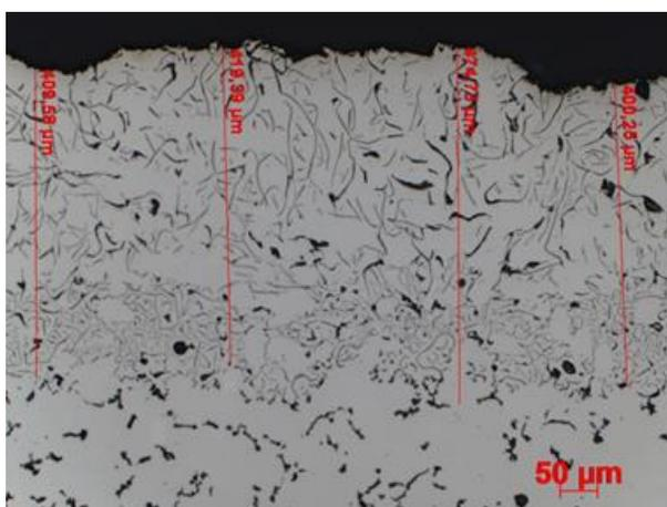
Fig. 6. Microstructure of casting made in moulding sand based on Reclaim 3 with sulphur content of 0.184%. Non-etched state
