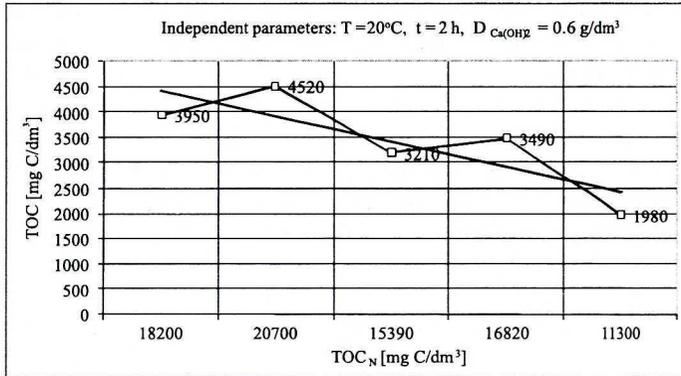
Fig. 13. Influence of total organic carbon value  $\text{TOC}_N$  in inflow wastewater on total organic carbon TOC value in wastewater after coagulation
