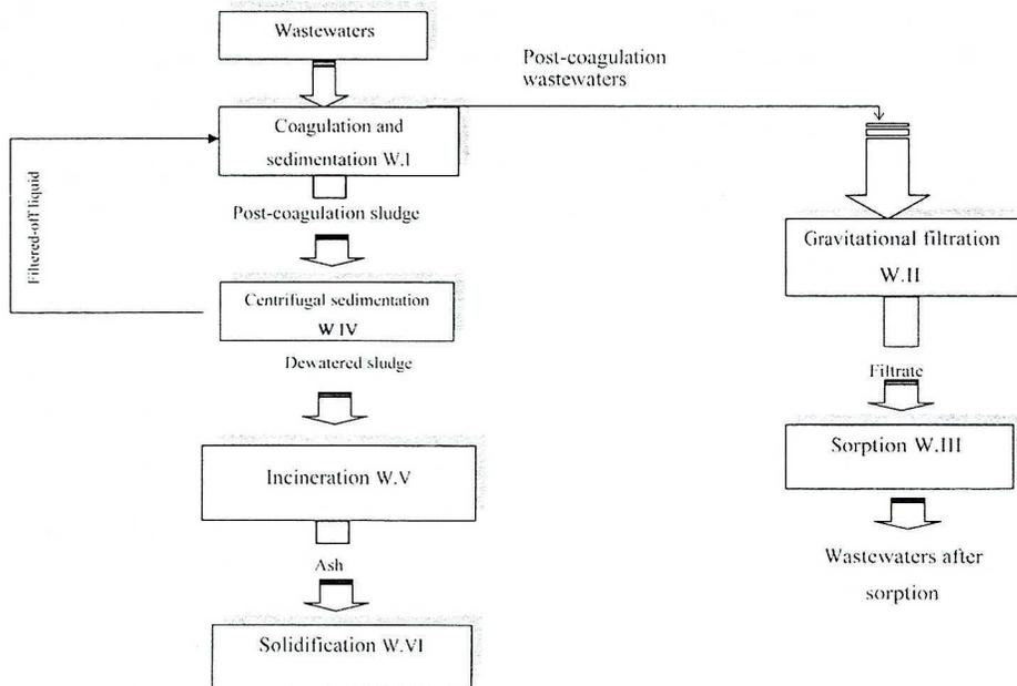
Fig. 1. Diagram presenting the treatment sequence for wastewaters from the DREWEXiM Company
