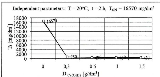
Fig. 2. Influence of  $\text{Ca}(\text{OH})_2$  dose on the concentration of total suspension  $T_s$  in wastewater after coagulation
