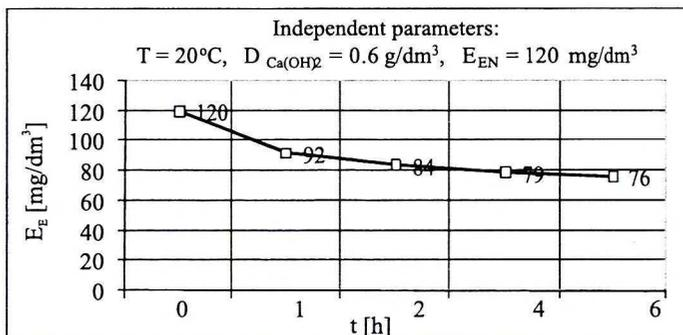
Fig. 9. Influence of sedimentation time  $t_s$  on ether extract value in wastewater after coagulation
