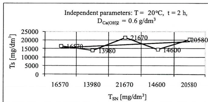
Fig. 4. Influence of the concentration of total suspension in inflow wastewater  $T_{\text{SN}}$  on the concentration of total suspension in wastewater after coagulation  $T_s$
