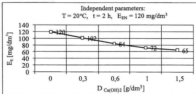
Fig. 8. Influence of  $\text{Ca}(\text{OH})_2$  dose on the ether extract value  $E_E$  in wastewater after coagulation
