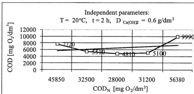
Fig. 7. Influence of COD value in inflow  $\text{COD}_N$  on COD value in wastewater after coagulation
