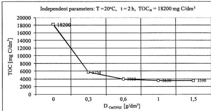
Fig. 11. Influence of  $\text{Ca}(\text{OH})_2$  dose on total organic carbon TOC in wastewater after coagulation
