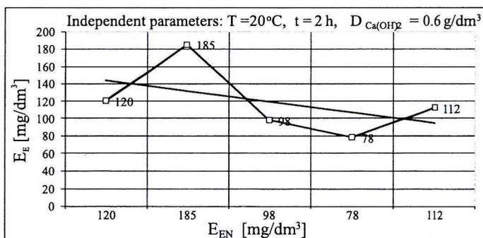
Fig. 10. Influence of ether extract value in inflow  $E_{EN}$  on ether extract  $E_E$  value in wastewater after coagulation
