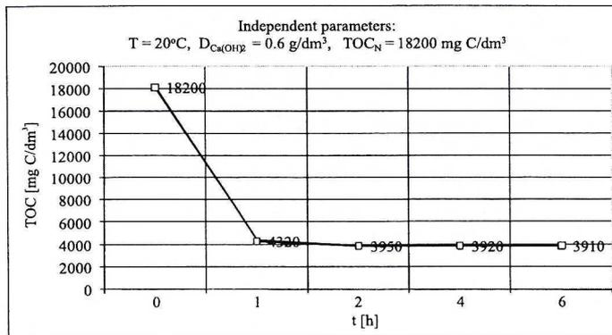
Fig. 12. Influence of sedimentation time  $t_s$  on the total organic carbon value TOC in wastewater after coagulation
