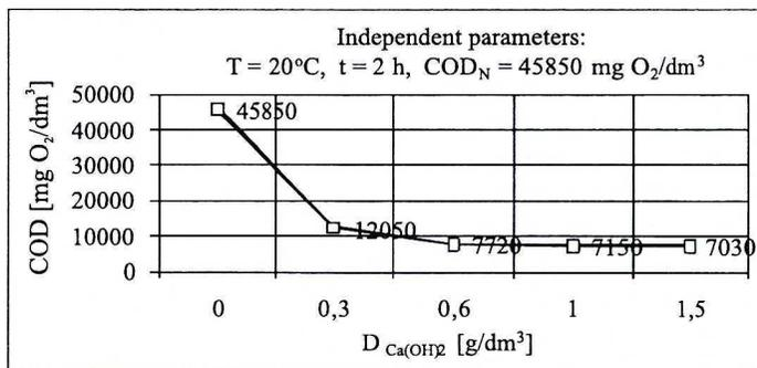
Fig. 5. Influence of  $\text{Ca(OH)}_2$  dose on the value of COD in wastewater after coagulation
