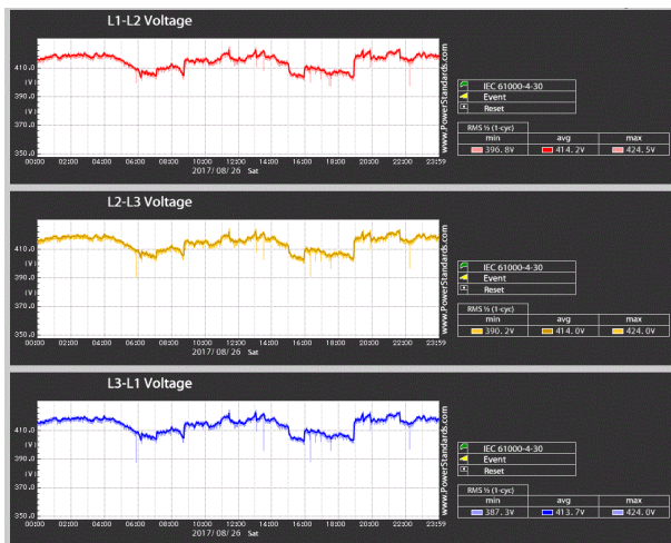
Fig. 1. Normal range of voltage during drive operation
