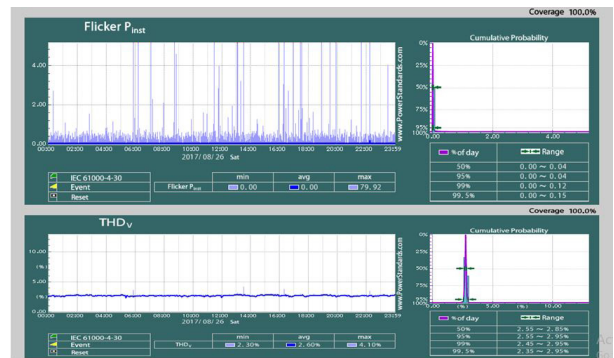
Fig. 2. Pretended voltage side harmonics and flickering effect during event non-occurrence phase
