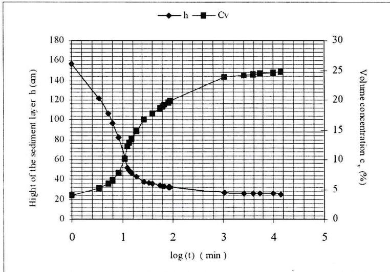
Fig. 4. Changes in volume concentration as a function of changes in the Odra River sediment layer height during sedimentation test
