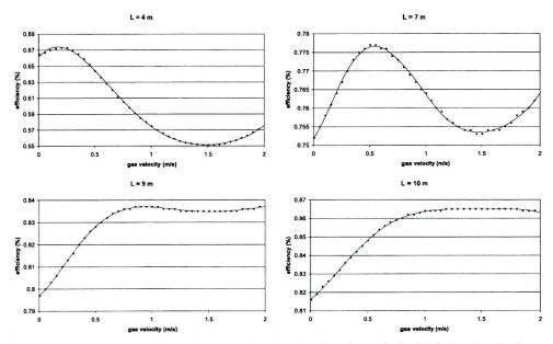
Fig. 6. The efficiency of the ESP in the middle of zone as a function of gas velocity  $(v_1)$  for L = 4 m, L = 7 m, L = 9 m and L = 10 m
