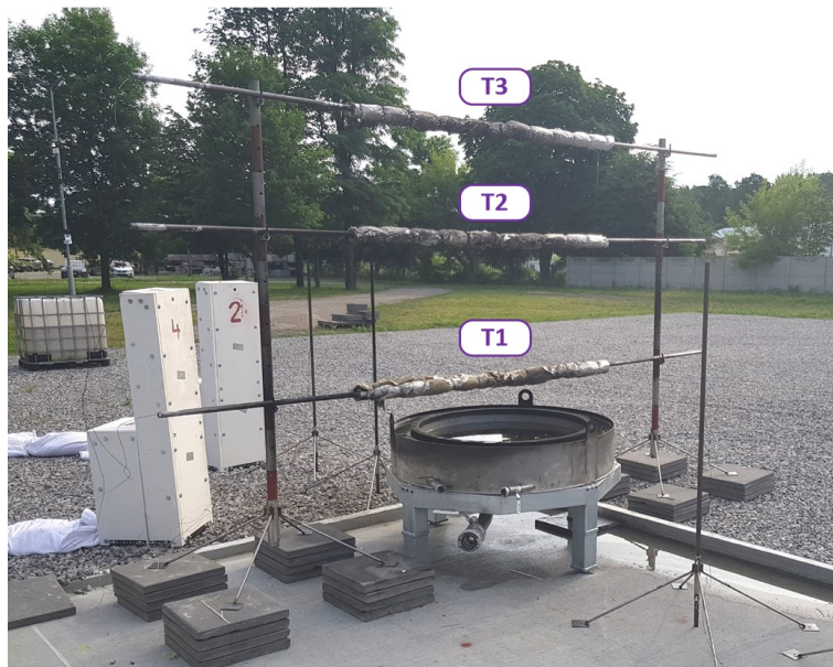
Fig. 1. Pool fire test stand: T1–T3 – thermocouples
