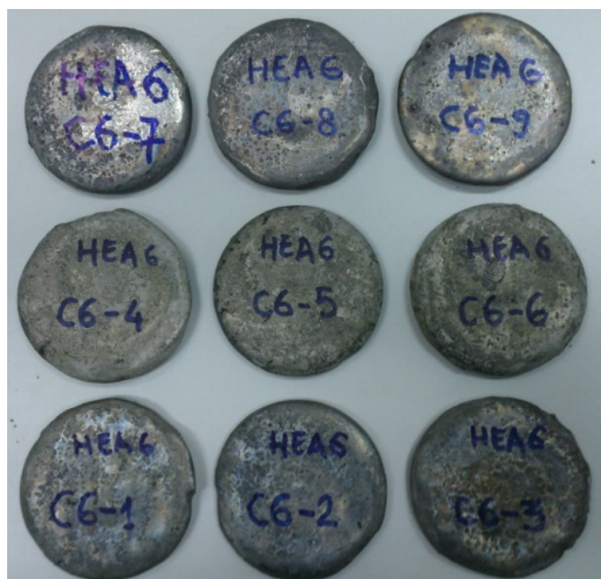
Fig. 1. As-cast HEA samples from AlCoCrFeNi alloying system
