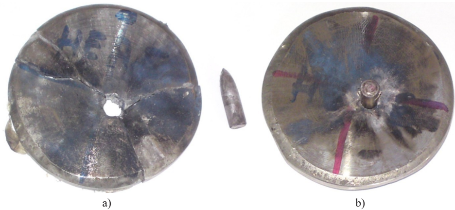
Fig. 5. The impact behaviour of HEA plates before and after heat treatment
