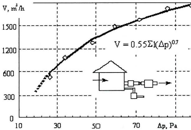
Fig. 10. Results of pressurization test in one of detached houses with new windows (for  $\Delta T \sim 15\text{K}$  and  $w < 0.8$  m/s)
