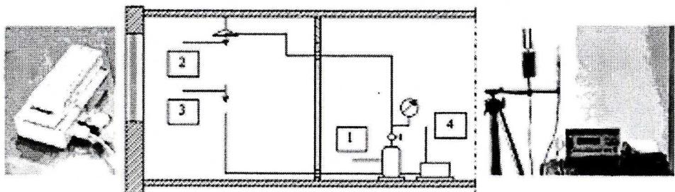
Fig. 5. Scheme of the measuring stand (a gas technique for flats and rooms)
