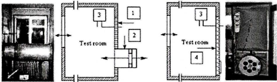
Fig. 3. The schematic diagram of large-scale pressurization test (for flats or rooms in BF and for offices in OB)
