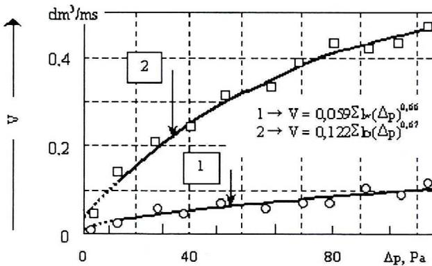
Fig. 6. Results of small-scale pressurization tests for windows (1) and doors (2)
