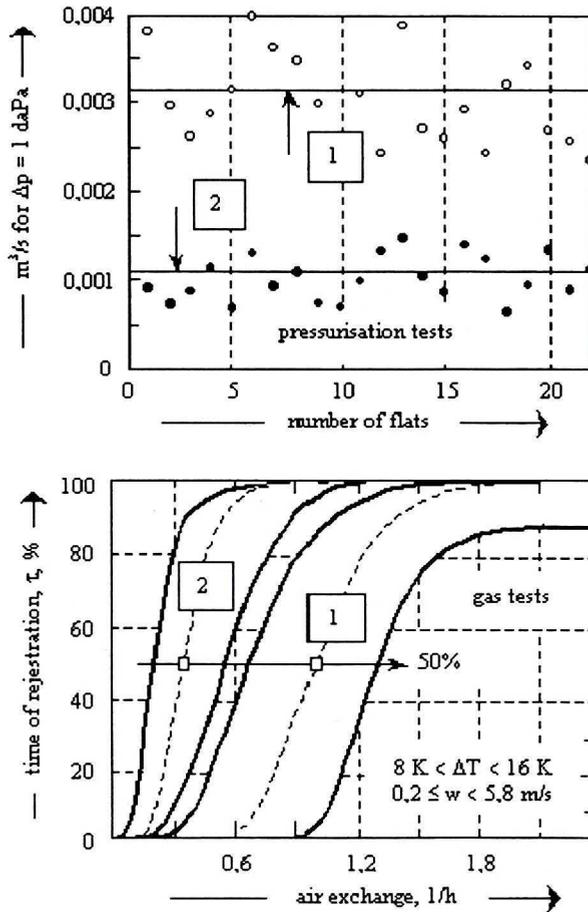
Fig. 7. Results of pressurisation (upper diagram – for:  $-2^{\circ}\text{C} < t_c < +10^{\circ}\text{C}$  and  $w < 4.2$  m/s) and decay of gas tests in one of examined block of flats
