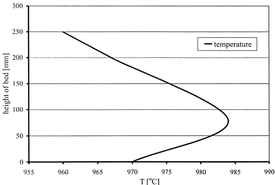
Fig. 2. Distribution of temperatures in the fluidized bed
