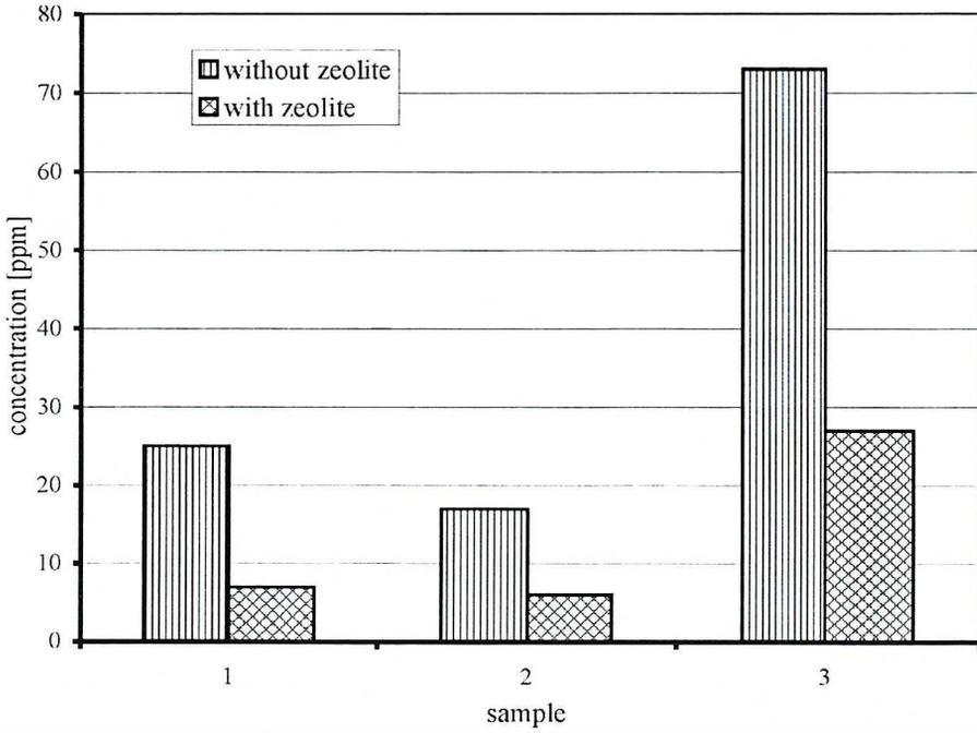
Fig. 6. NO concentration reduction in fluidized combustion
