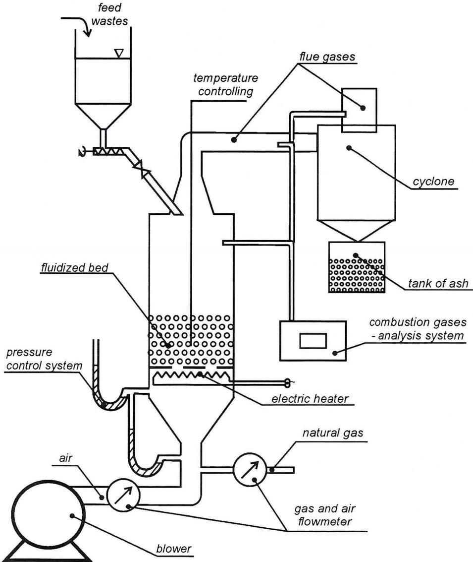
Fig. 1. Flow sheet of experimental apparatus for fluidized bed combustion technology
