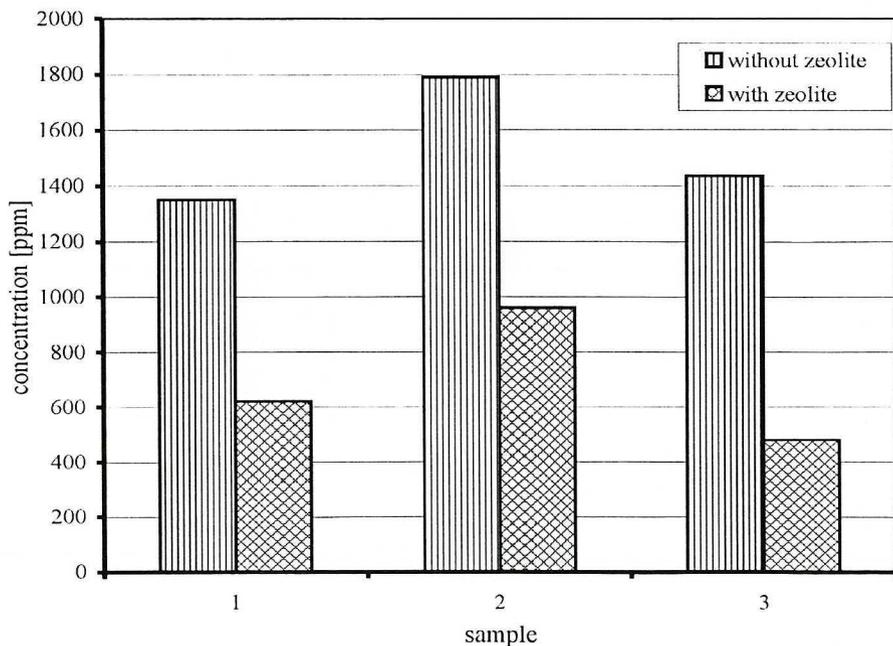
Fig. 5. CO concentration reduction in fluidized combustion
