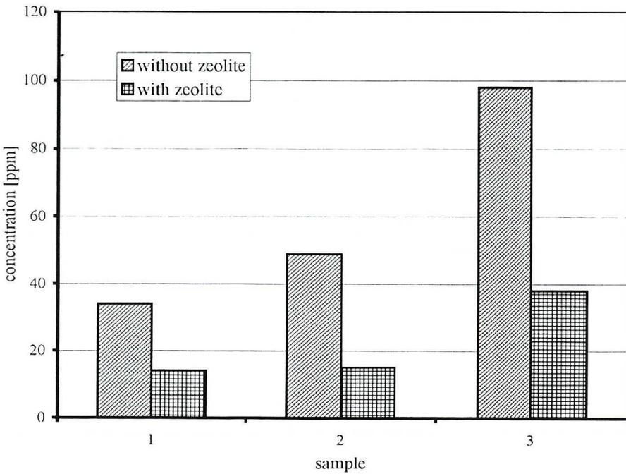
Fig. 7. SO<sub>2</sub> concentration reduction in fluidized combustion
