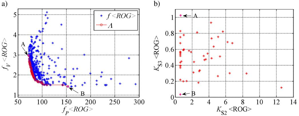
Figure 3: Values of the components of the objective function ( $\mathbf{f} \langle \text{ROG} \rangle$ ) and the set of compromises  $\Lambda$  (a) and the optimized power stabilizer parameters  $K_{S2}$  and  $K_{S3}$  corresponding to the compromise set (b) for polyoptimization of PSS in the generating unit ROG411
