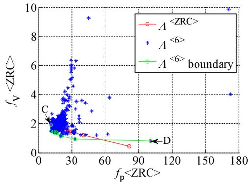
Figure 12: Comparison of the six-dimensional set of compromises  $\Lambda^{<6>}$  and its two-dimensional boundary  $\Lambda^{<6>}$  boundary with the two-dimensional set of compromises  $\Lambda^{<ZRC>}$  on the plane  $f^{<ZRC>}$
