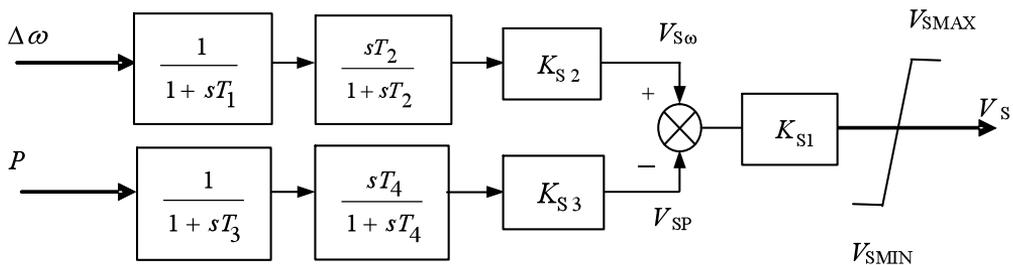
Figure 1: Structural diagram of the dual-input stabilizer PSS3B
