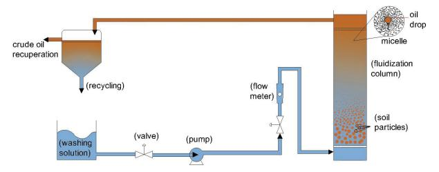
Fig. 2. Schematic representation of laboratory experimental setup
