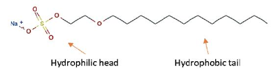
Fig. 1. The chemical structure of SLES (SLES)
