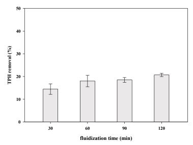
Fig. 3. Variation of TPH removal ratio with time (free water washing)
