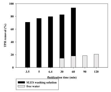
Fig. 5. The effect of fluidization time on TPH removal rate for free water and surfactant solutions
