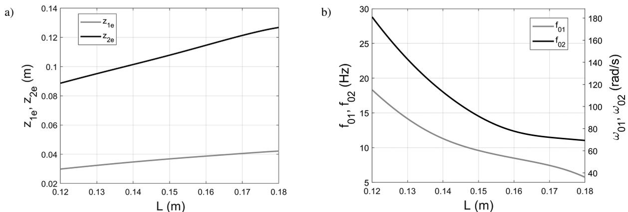
Fig. 3. Changes in equilibrium positions (a) and linear natural frequencies ( $\omega_0 = 2\pi f_0$ ) (b) versus distance  $L$
