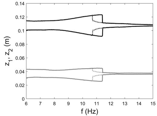
**Fig. 7.** Characteristics of maximum and minimum values of system responses. Simulations made with the constant excitation acceleration amplitude of 0.6g. Solid line – forward frequency, dashed line – backward frequency, gray line –  $z_1$ , black line –  $z_2$
