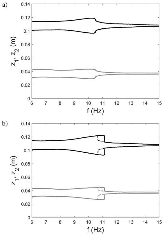
**Fig. 9.** Characteristics of maximum and minimum values of system responses. Simulations were made with the constant excitation acceleration amplitude of 0.6g and resistances a)  $R_1 = R_2 = 2000 \Omega$  and b)  $R_1 = R_2 = 10000 \Omega$ . Solid line – forward frequency, dashed line – backward frequency, gray line –  $z_1$ , black line –  $z_2$
