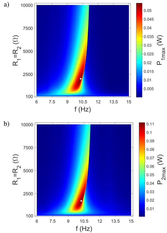
**Fig. 12.** Color maps showing the maximum  $P_1$  (a) and maximum  $P_2$  (b) versus resistance and excitation frequency. The maps were obtained with forward frequency sweep and 0.6g excitation amplitude. The white point marks the global maximum
