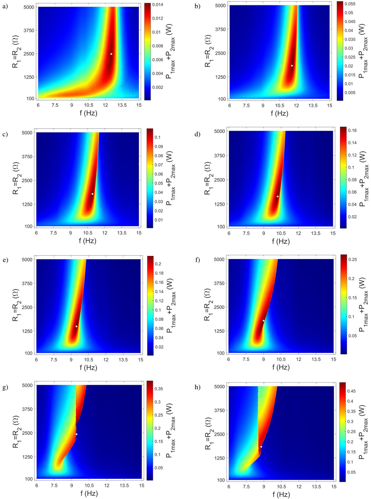
**Fig. 13.** Color maps showing the sum of maximum  $P_1$  and maximum  $P_2$  versus resistance and excitation frequency when  $L$  is equal to: 0.135 m (a), 0.14 m (b), 0.145 m (c), 0.15 m (d), 0.155 m (e), 0.16 m (f), 0.165 m (g), 0.17 m (h). The maps were obtained with forward frequency sweep and 0.6g excitation amplitude. The white point marks the global maximum
