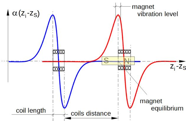
**Fig. 8.** Examples of curves of electromechanical coupling coefficient versus magnet position in relation to the coils. The coupling between magnet and right coil (red), the coupling between magnet and left coil (blue)
