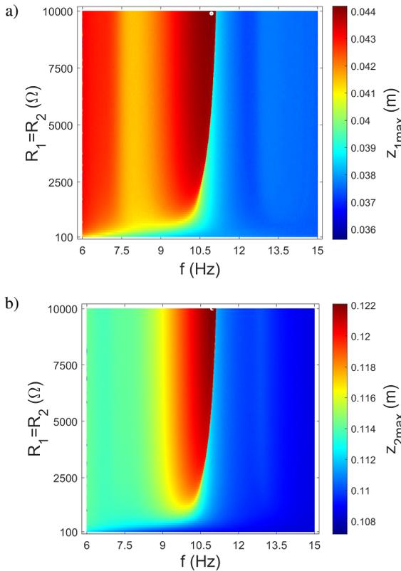
**Fig. 11.** Color maps showing the maximum  $z_1$  (a) and maximum  $z_2$  (b) versus resistance and excitation frequency. The maps were obtained with forward frequency sweep and 0.6g excitation amplitude. The white point marks the global maximum
