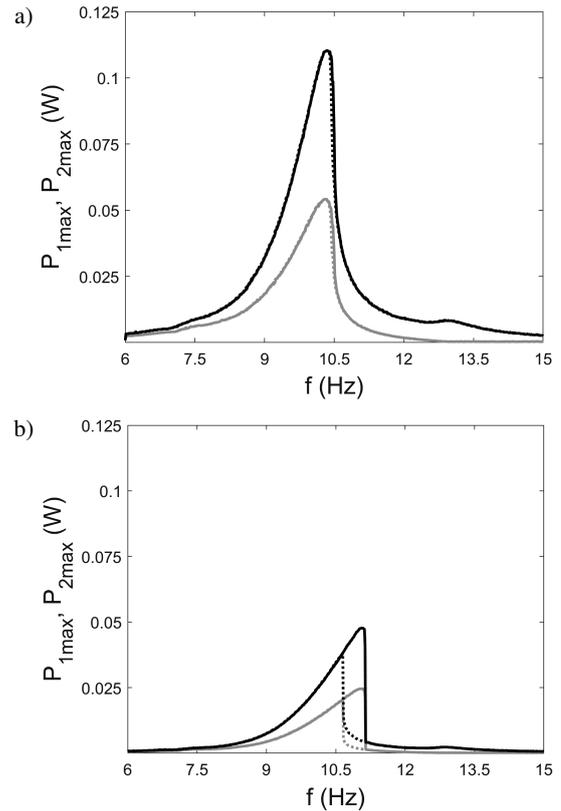
**Fig. 10.** Characteristics of maximum values of power recovery energy. Simulations were made with the constant excitation acceleration amplitude of 0.6g and resistances a)  $R_1 = R_2 = 2000 \Omega$  and b)  $R_1 = R_2 = 10000 \Omega$ . Solid line – forward frequency, dashed line – backward frequency, gray line –  $P_1$ , black line –  $P_2$
