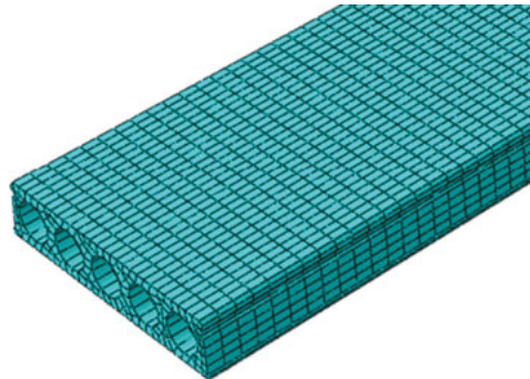
Fig. 6. Discretization of the hollow-core slab PHC 26.5-6
