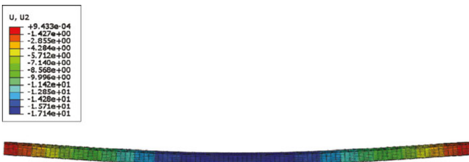
Fig. 14. Vertical displacement of the plate PHC 40.0-9 due to prestress and external load [mm]
