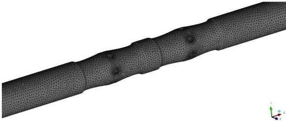
(b) Prism grids near the tube wall
