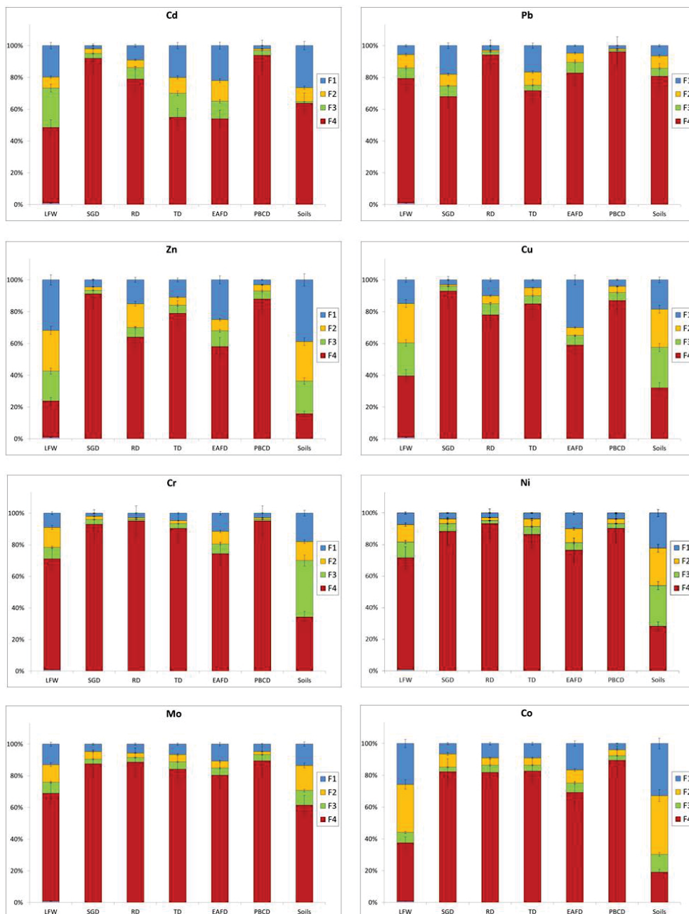
Fig. 1. Speciation analysis of waste and soil samples according to SM&T procedure LFW – landfilled foundry waste; SGD – shock grating dust; RD – e-generation dust; TD – transport (of molding sands) dust; EAFD – electric arc furnace dust; PBCD – pneumatic blast cabinet dust; F1–F4 – fractions of SM&T procedure
