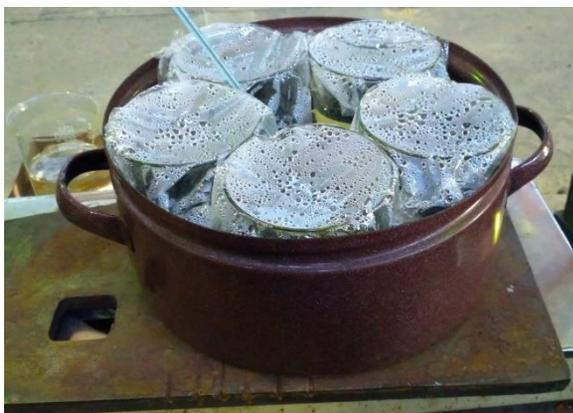
Fig. 3 Test apparatus in temperature  $55 \pm 7$  °C
