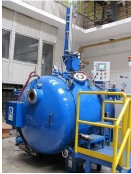
Fig. 2. The Seco-Warwick VIM-20 vacuum induction melting furnace
