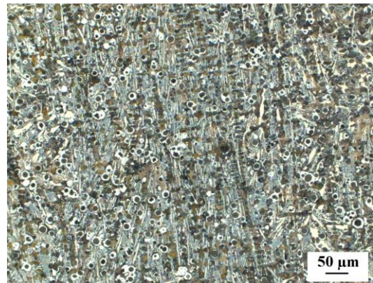
Fig. 1. Microstructure of cast iron used in the test, metallographic specimen etched in the Mi1Fe reagent (4% Nital), LM, microscope magnification 200x
